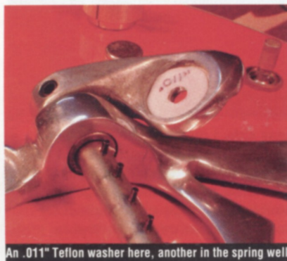
An .011" Teflon washer here, another in the spring well
