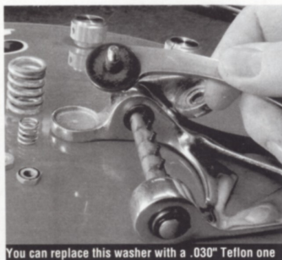
You can replace this washer with a .030" Teflon one
