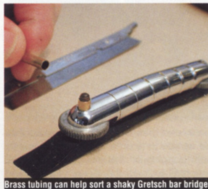
Brass tubing can help sort a shaky Gretsch bar bridge
