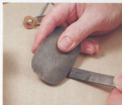
Finally, any high spots can be removed for a perfect fit
