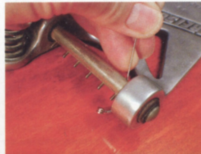
Pre-curve your string-ends for hassle-free stringing
